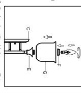
Step.3: Put the glass (G) with the covers (F) into the cup (E).Use Max 60W bulb.
